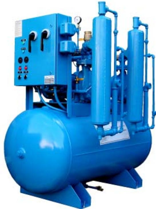
Externally operable circuit breakers with a door interlock, control circuit transformers with fused primary and secondary coils, H-O-A switches, magnetic starters with 3 leg overload protection and reset switches are standard. The Programmable Logic Controller provides automatic alternation and lead-lag control with the option to select either one of the pumps as a permanent lead for periods of pump maintenance. It includes minimum run timers to prevent short cycle operation.
