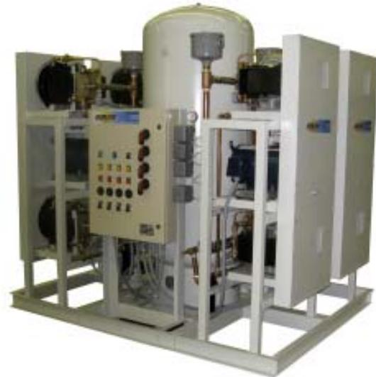
The dryer is designed to provide a maximum dew point below +32°F per NFPA 99. Built-in purge saver control automatically minimizes the amount of purge air to match the variable airflow.
