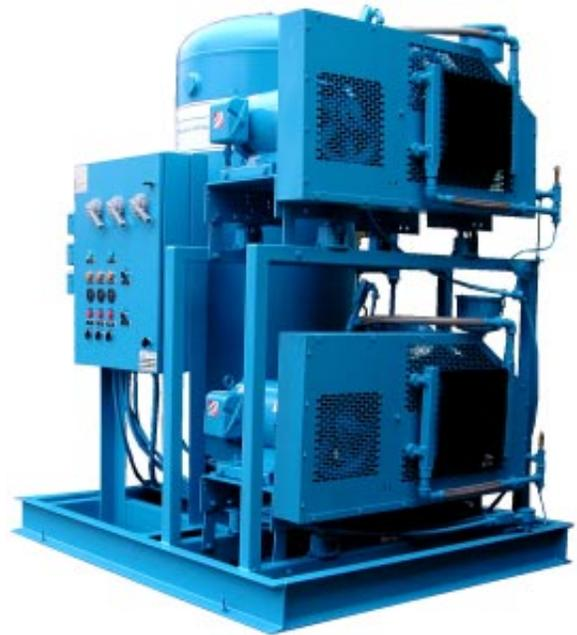
The visual alarm remains energized until the problem is corrected. Each alarm function includes a set of dry contacts for connection to the master alarm. All control and alarm functions remain energized while any compressor in the system remains electrically on-line.
