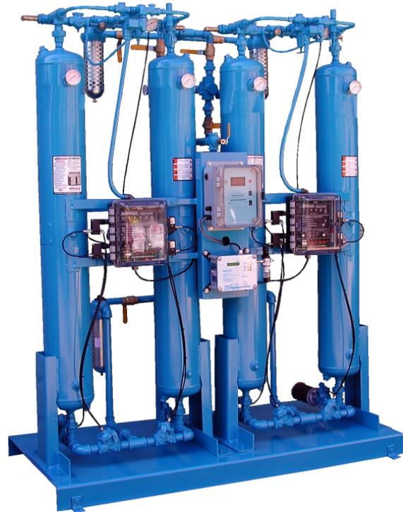
Digital dew point and CO monitors with alarm set points at  $39^{\circ}\text{F}$  and 10 PPM are provided.
