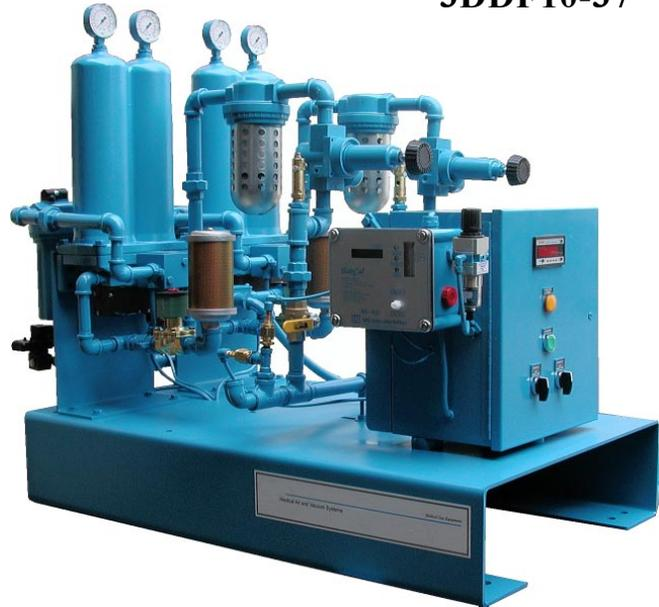
Downstream pressure regulators equipped with pressure indicators will maintain constant delivery pressure of 55 PSIG plus or minus 10% (field adjustable).
